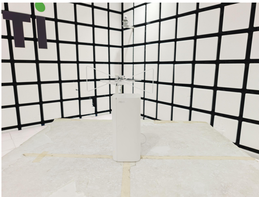
Radiated spurious emission Test Setup-1(Below 1GHz)
